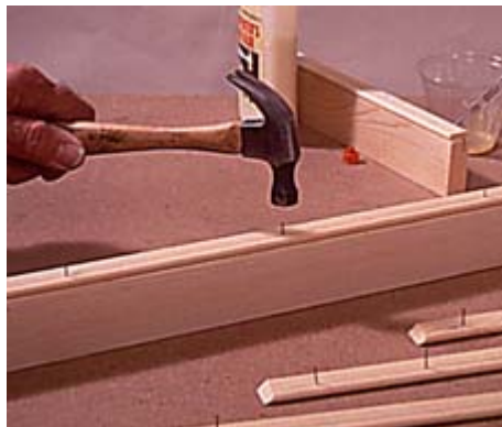
15 --Make the beading from 1/4-in. lattice. Cut the round edge with a 1/8-in.-rad. half-round bit mounted in a router table.
