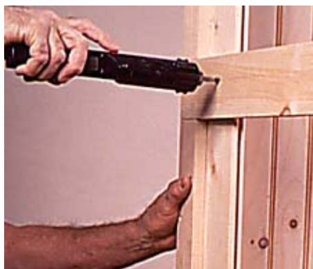
5 --Attach L-shaped pieces to side to facilitate clamping side to stile. When the glue has cured, scrape away excess.
