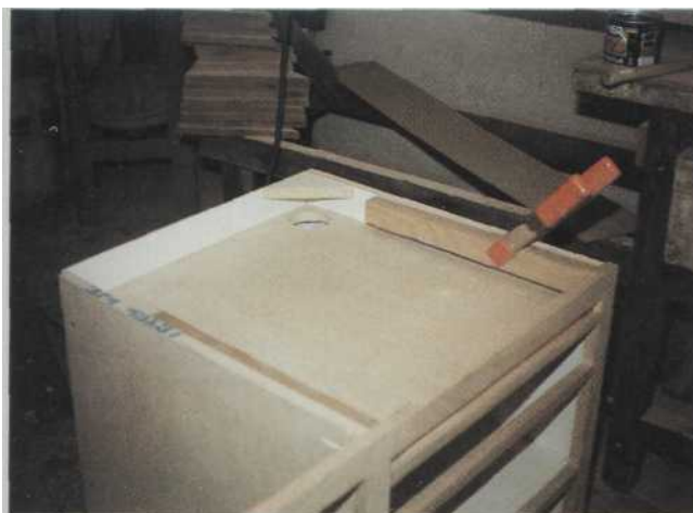
4 The pull out board is shown in place with a top guide (V) being held in place with squeeze clamps.
