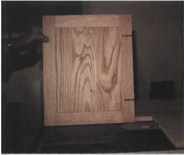
8 The back of the door shows the dadoes cut to receive the hinges.
