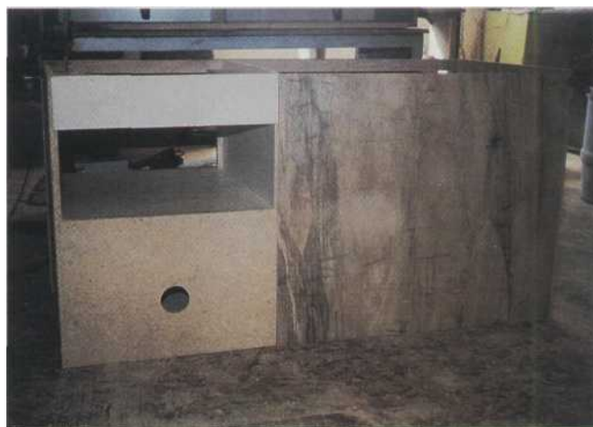
3 The three backs in the desk unit shown in place. Notice the wire chase hole for the printer drawer.
