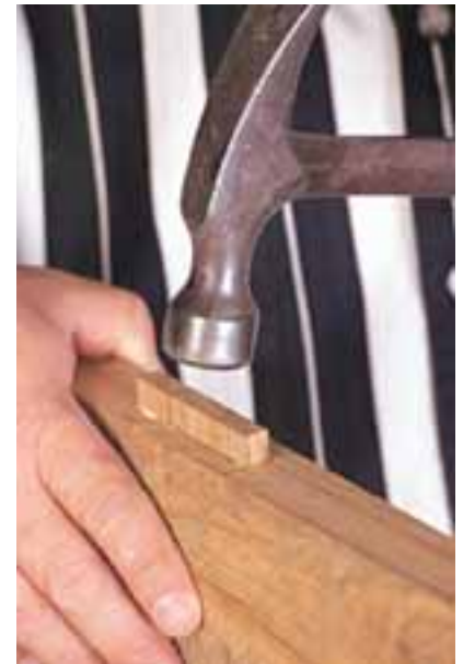
The plugs for the breadboard ends are made from the same material as the table top. Sand the plug to fit, put some glue on the sides and tap it in place.
