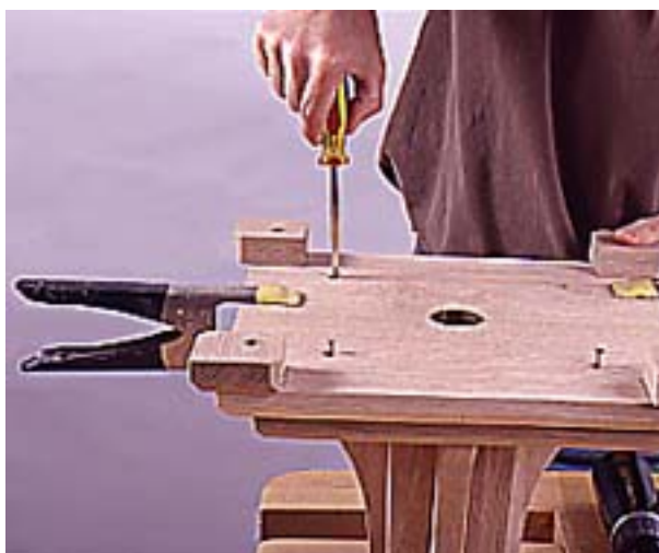
8--Cut the feet and lower base to size. Then attach the feet and join the two base pieces with glue and screws.
