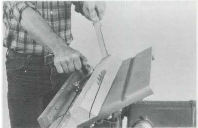
Triangle formed by saw kerf and blade should be \frac{3}{4} " on each side. (Saw guard removed for clarity only.)
