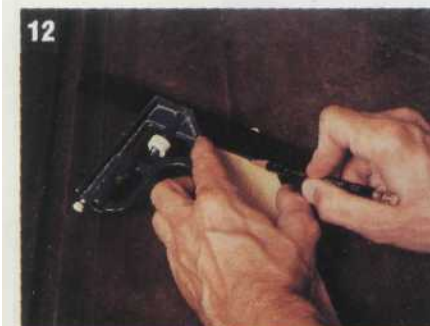
12 Mark the miter lines on one end of each of the four remaining 1" x 1 3/4" x 18" border strips.
