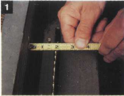
1 Set the table saw blade at a 90° angle and measure exactly 1 3/4" from the fence.
