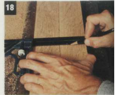
18 Use a square to carry the mark to the adjacent piece, then cut both. Repeat the procedure on the remaining pieces to make four 19" leg blanks.
