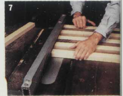
7 After 24 hours, once the glue is dry, square up the board against the miter gauge and carefully trim the squared edge.
