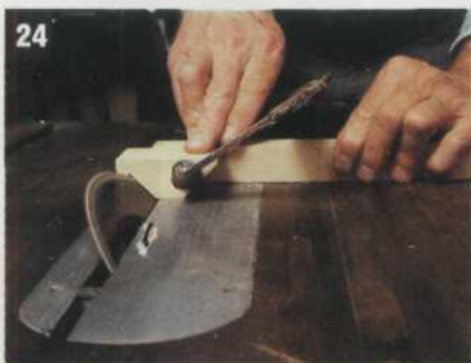
24 Tilt the table saw blade to a 45° angle and cut the four 1" x 1¾" x 2½" corner braces. Because the work is so close to the blade, clamp each brace to a scrap of 1 x 2 and make the cuts that way. Be sure the clamp clears the blade before starting the saw.
