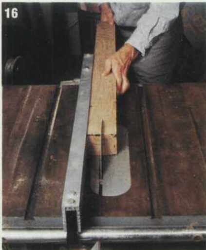
16 Rip the 2" x 3" x 40" leg billet in half to make two 1½" x 2" x 40" pieces.
