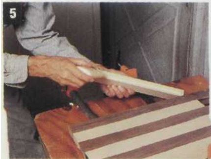
5 Glue the strips together with an even bead, alternating the four dark and five light species to make a 15 3/4" width. Place the best face down toward the clamps.
