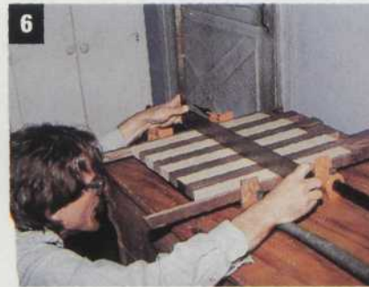
6 Use the edge of a framing square to check the plane of this initial glue-up. Any inconsistencies should show on the exposed side, which will be the underside of the table surface. Square one edge as well before tightening the clamps.
