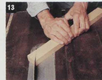
13 Establish the exact length of the first piece against one edge of the board and mark the opposite miter. Set the miter gauge to a 45° angle, and cut the first border piece. Cut the marked ends of the other three pieces.
