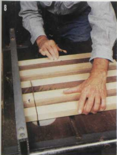
8 Reset the fence for a 1¾" cut and pass the board through the blade until you've got eight dark-and-light strips. Arrange them in the same order they've been cut.
