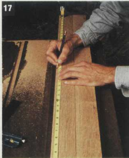
17 Lay the pieces side by side, align the ends flush, and mark at 19".
