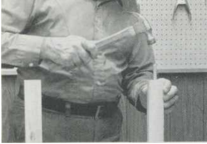
The frame sections of the china hutch are assembled with the aid of glue and spiral dowels. Dowel centers are recommended to
