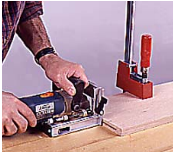
5--Clamp the bottom shelf securely to a workbench. Then use a plate joiner to cut joining slots in both ends of the shelf.
